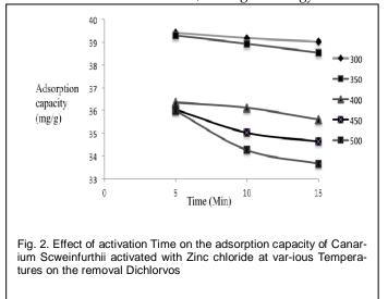
rated and adsorption begins at low energy site which result in a decreases in adsorption efficiencies [13]. The low removal efficiency of the activated carbon with increase in activation time can be explained in term of insufficiency of micropore structure formation with increased time of activation.
